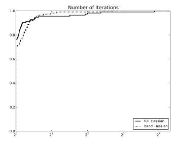
Figure 1: Performance profile in terms of number of iterations comparing P = band(H) with P = H in (80).
